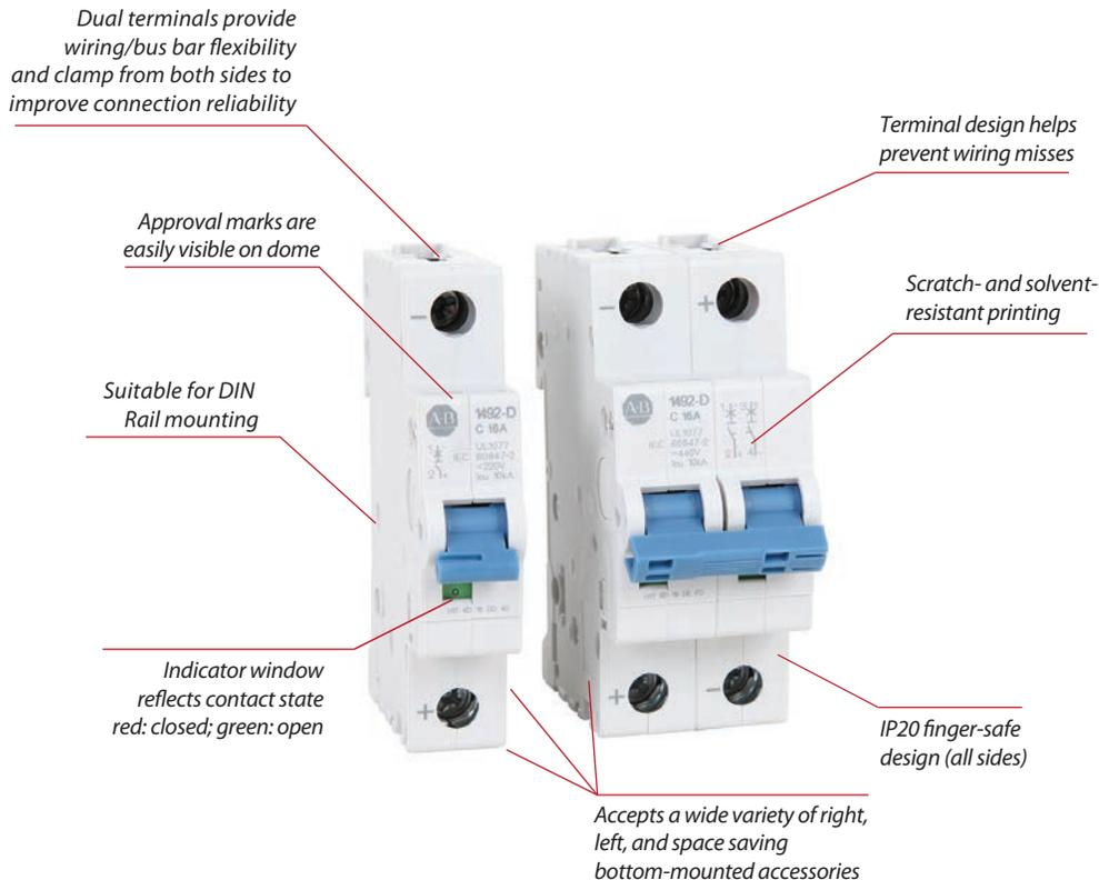
Bulletin 1492-D Miniature Circuit Breakers provide overcurrent and short circuit protection for higher voltage DC circuits. These devices are also Miniature Circuit Breakers as defined by IEC Standards.
